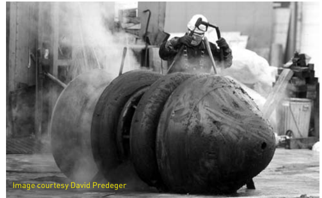
Image courtesy David Predeger A TAPS employee cleans a scraper pig at the Valdez Marine Terminal. Scraper pigs, which clean the pipeline and enhance oil flow, are pushed by the oil.
