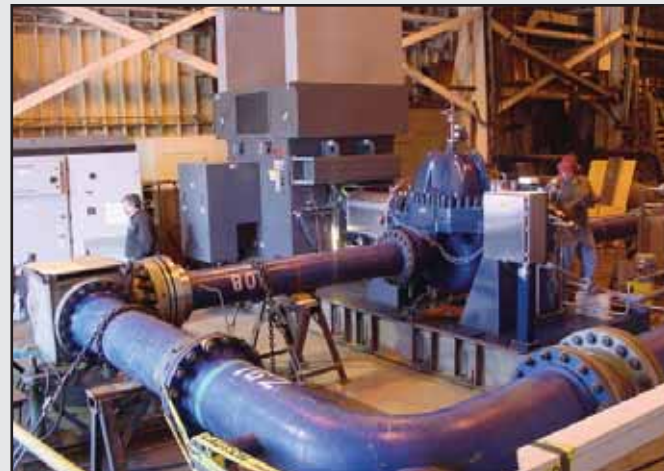
Each operating pump station will house three Sulzer two-stage centrifugal pumps. Each pump will be driven by a 6,500-horsepower electric motor. The two photos below show the crude pump connected to the electric motor during a test at Sulzer's plant in Portland, Oregon.
