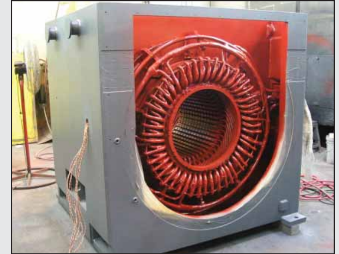
The electric motors being installed in the pump modules have large square housings. The red rings in the center are the windings for the motor. This is the "stator", which remains stationary while the motor is in operation. The magnetic field in the stator creates an opposing magnetic field in the "rotor" to make the rotor spin. These motors run off 6,300-volt electrical power.
