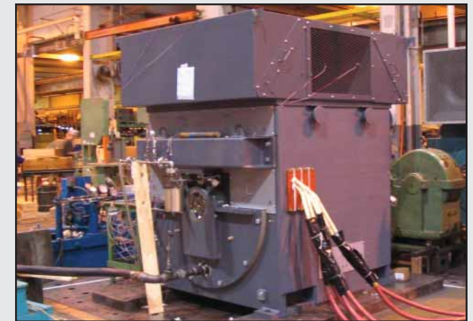
The electric motors being installed in the pump modules have large square housings. The red rings in the center are the windings for the motor. This is the "stator", which remains stationary while the motor is in operation. The magnetic field in the stator creates an opposing magnetic field in the "rotor" to make the rotor spin. These motors run off 6,300-volt electrical power.
