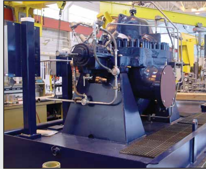
Each operating pump station will house three Sulzer two-stage centrifugal pumps. Each pump will be driven by a 6,500-horsepower electric motor. The two photos below show the crude pump connected to the electric motor during a test at Sulzer's plant in Portland, Oregon.
